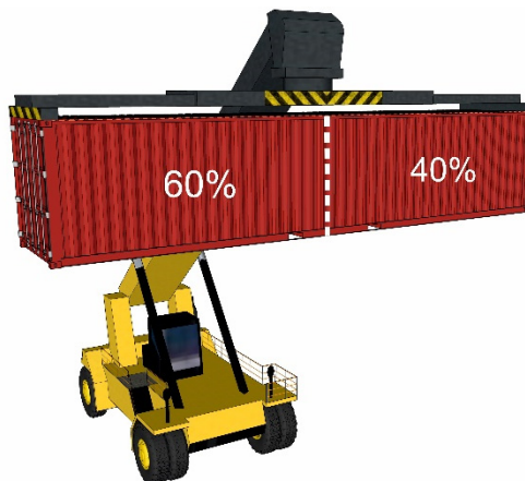
Weight distribution in a container
