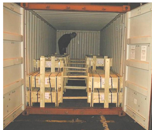
Blocking with timber
