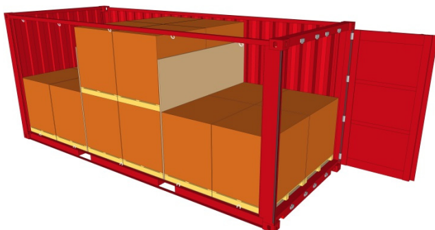
Threshold created by using cargo units with different heights
