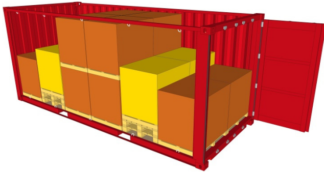
Threshold created by using empty pallets under cargo units with the same height
