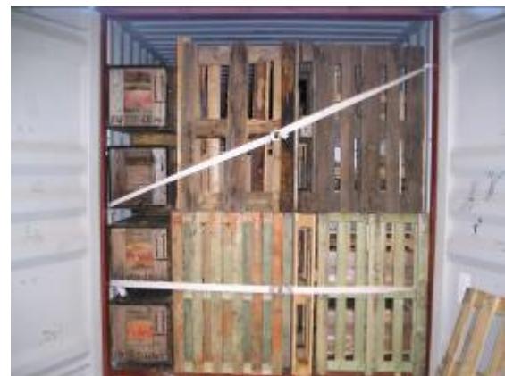
Blocking with empty pallets
