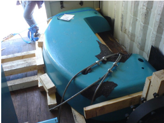
Blocking of machinery parts with timber
