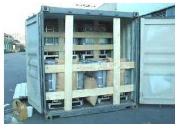
Blocking with dunnage bags and timber
