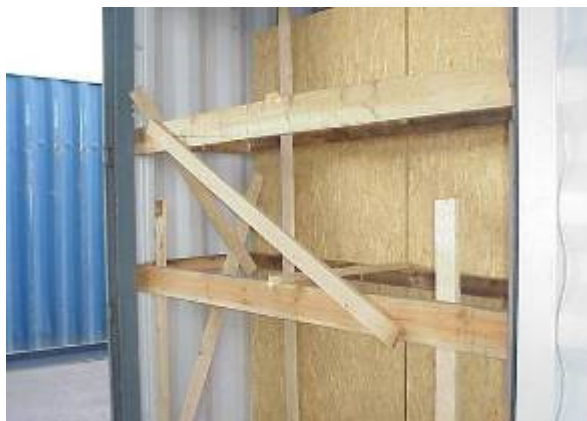
Blocking with timber
