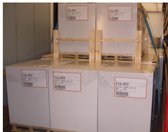
Upper layer blocked with boards and battens
