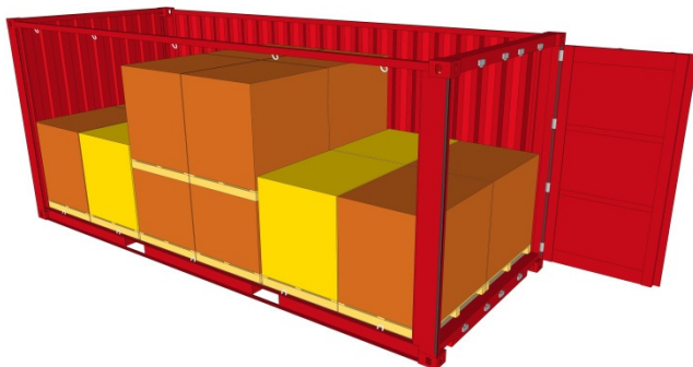
Threshold created by using empty pallets under cargo units with the same height
