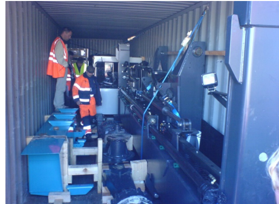
Blocking of machinery parts with timber
